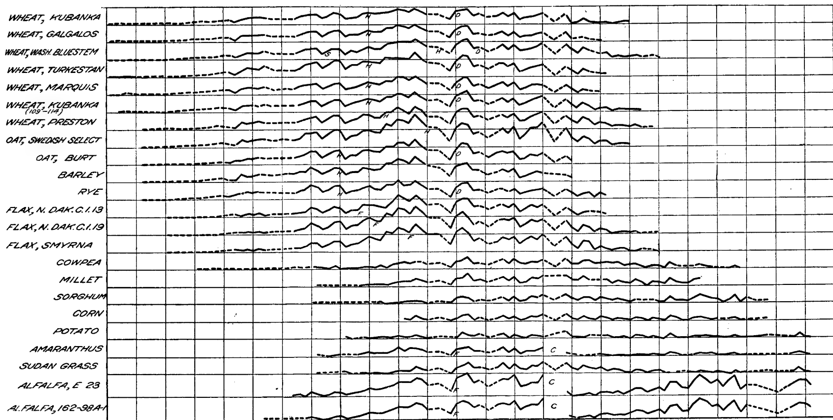
FIG. 3.—Graphs showing the daily intensity of environmental factors and the daily transpiration of 23 crops for the year 1915. The evaporation from the small tank is expressed in kilograms per square meter. The evaporation from the large tank is given in millimeters. The temperatures are expressed in degrees centigrade; the total radiation for the day in small calories per square centimeter on a surface normal to the sun's rays; the wet-bulb depression in hour degrees C.; the wind velocity in meters per second. The transpiration is given in kilograms, the space between the base (zero) lines for each crop representing 3 kgm., except for alfalfa, the base line of which is 5 kgm. below that of the crop above. The letter C in the graph indicates that the crop was cut and was followed by a new growth from the established root system. S signifies that the plants were forming shoots; H , heading; F , flowering; and D , lower leaves dying.
